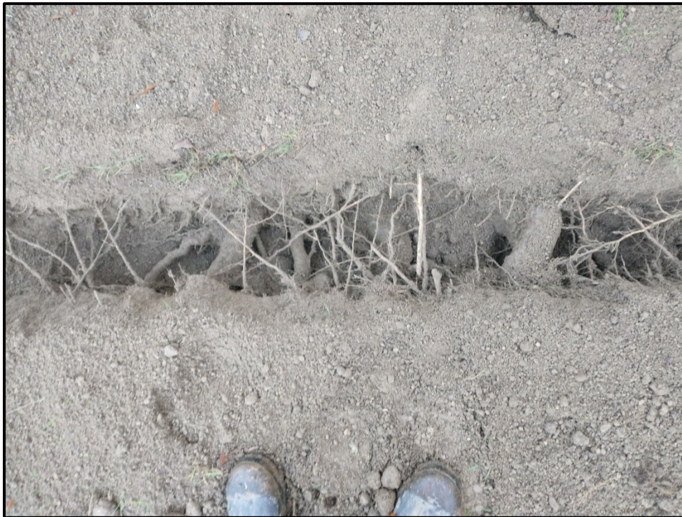
Photograph 2. Tree 13 trench with some structural roots encountered, although most roots were fine roots, or less than 1 inch in diameter.
